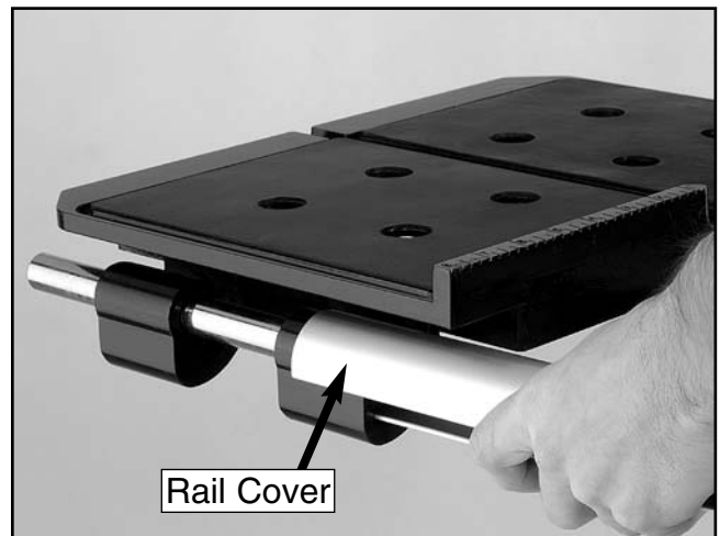
Figure 14. Assembling the rail cover.
